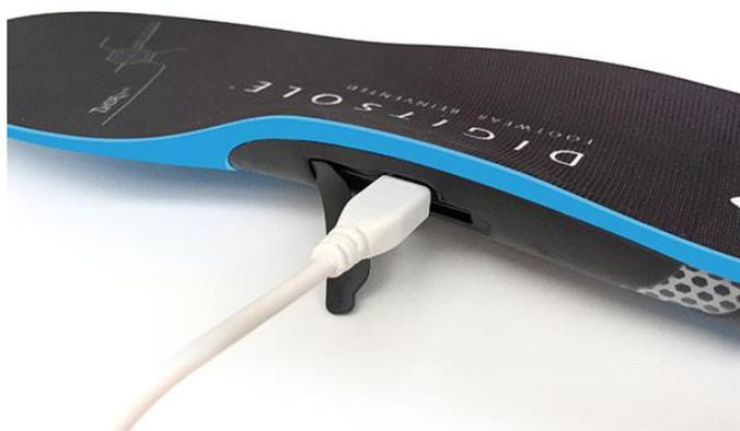
A full charge takes 2.5 hours. Once charged, the insoles can last up to seven days. The battery's lifespan varies depending on the use.
